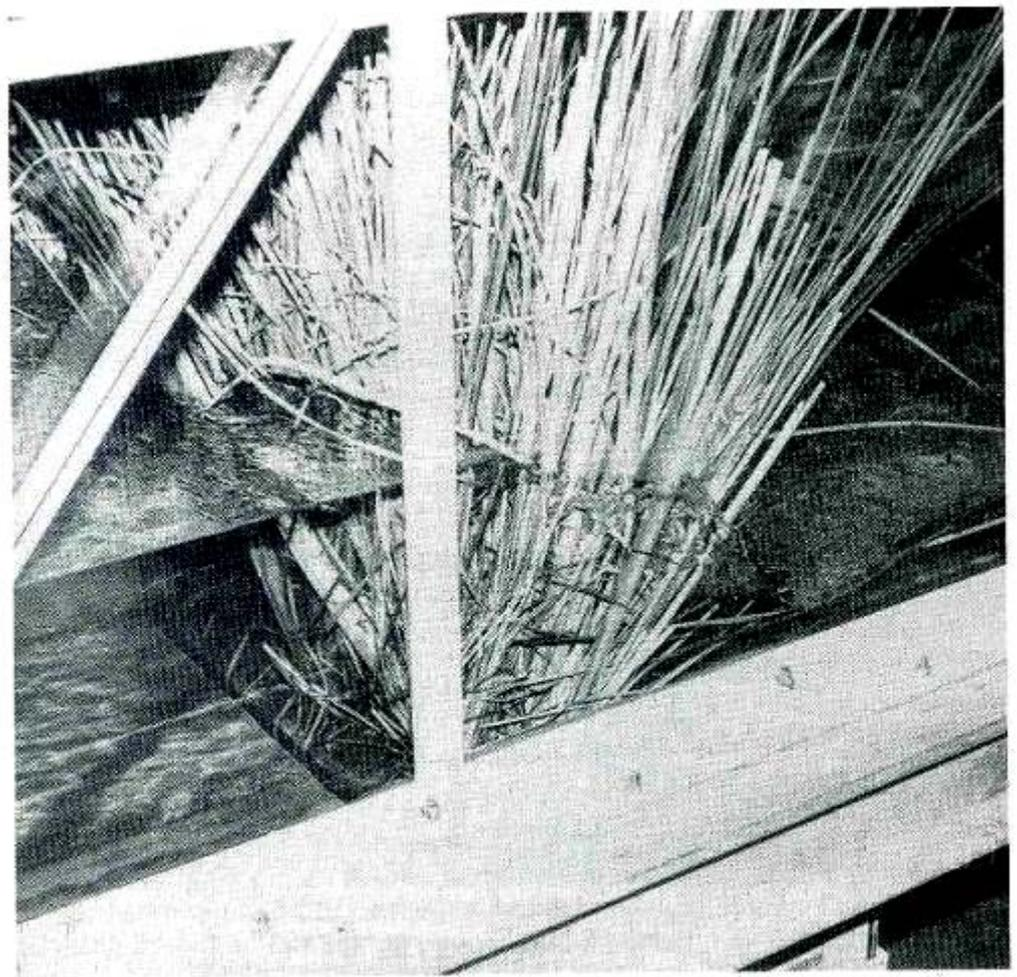
Oxford, Mississippi. In a recent trial, plant hedge held back water almost as if it were a dam. This test was conducted in a flume (61 cm wide) and the water (flowing at 28 liters per second) was ponded to a depth of 30 cm behind the hedge. This result was all the more remarkable because the hedge was young and less than 15 cm thick. (Sedimentation Laboratory, Agricultural Research Service, U.S. Department of Agriculture)
